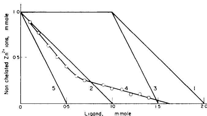
FIG. 1.—Amperometric titrations of 1:1 mixture of zinc and calcium ions with TTHA.
